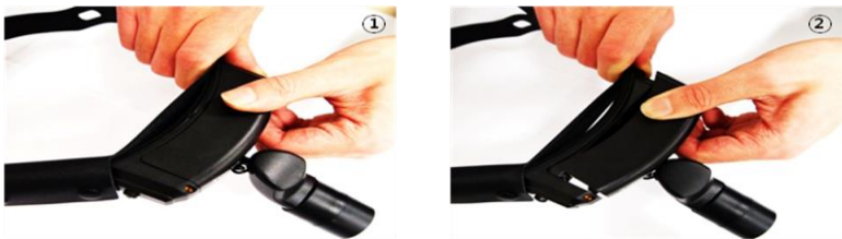
Fig. 3.2 Battery pack separation method
