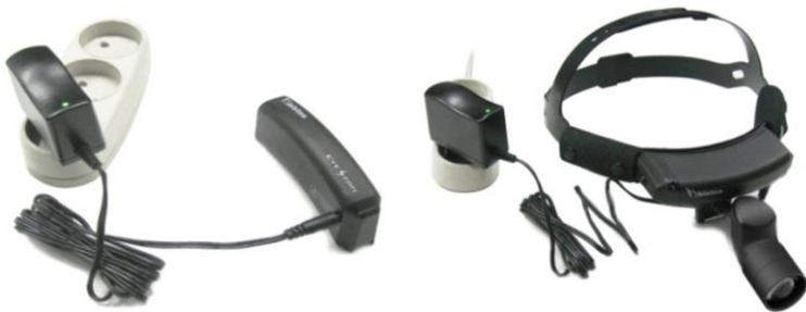
Fig. 3.3 Two way of charging the battery pack
